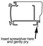
As you release the brackets, support the headrail to keep it from falling.
