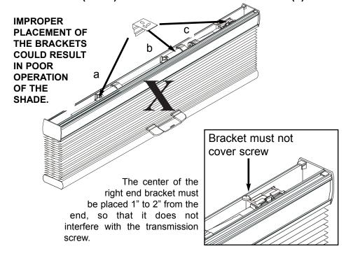
Using the Installation Bracket as a template, measure to the edge of the bracket and mark the hole locations with a pencil for drilling. When mounting brackets, make sure they are in line and level.
